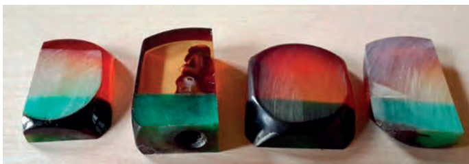
Figure 3. Oxidation means this car gear stick knob appears to be a dark cherry colour. However, cut into segments the true colour of the material is revealed as green with a translucent yellow top.
